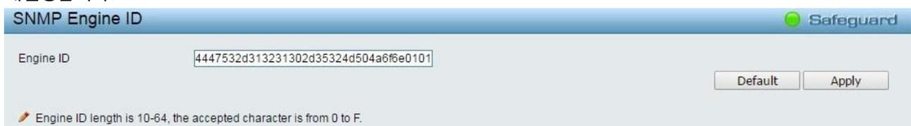
The screenshot shows the 'SNMP Engine ID' configuration page. It includes an 'Engine ID' input field containing the hexadecimal string '4447532d313231302d35324d504a6f6e0101'. There are 'Default' and 'Apply' buttons. A note indicates that the Engine ID length is 10-64 characters, and the accepted characters are from 0 to F.
